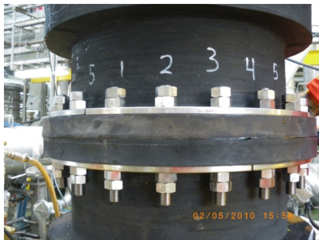
Fig. 17: Flange Connection with Super Duplex Studbolts & Nuts (No Anodes)
