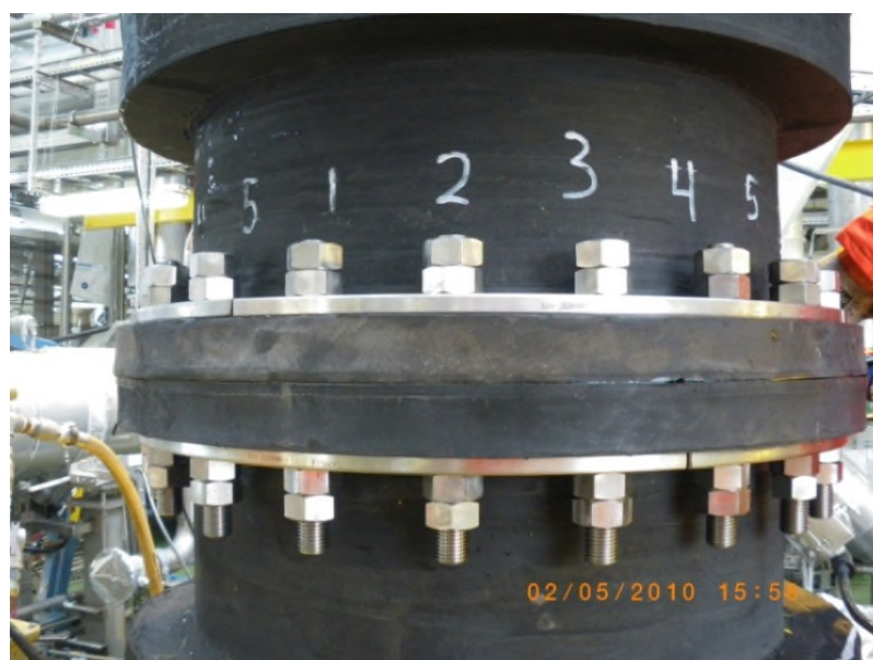
Fig.2-16: Flange Connection with Super Duplex Stud bolts (No Anodes)
