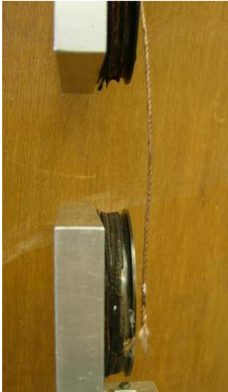
Figure 3 the failed 25% UBL specimen showing failure just outside the gauge length
