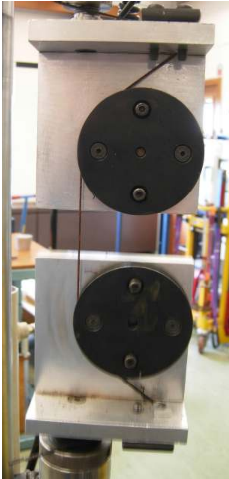
Figure 2 Set up for the Yarn Testing
