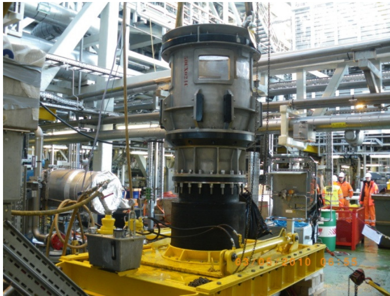
Riser Head: Manufactured from 6Mo HDPE Seat / Pads at contact points
