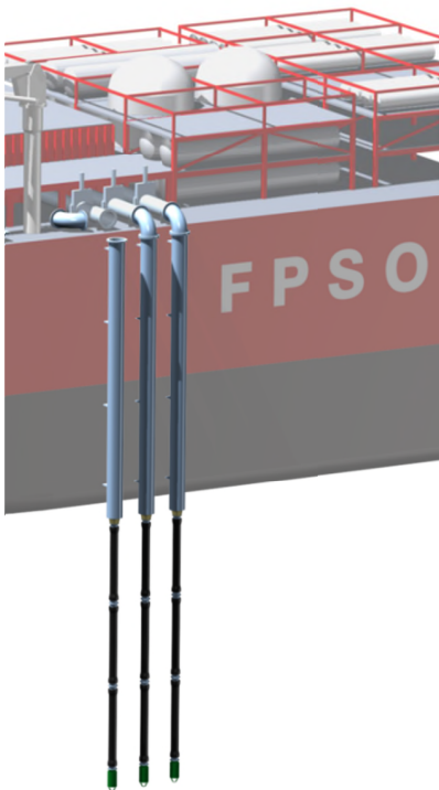
Fig 1.: Typical Seawater Intake Riser (SWIR) Arrangement on FPSO
