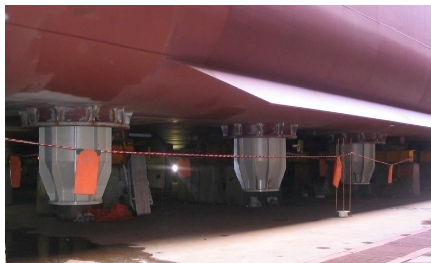
Fig.2-21: Vessel fitted with Internal Caissons (and riser heads in trial fit)
