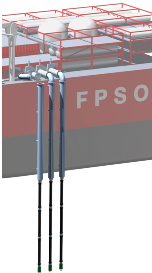
Fig. 3: Typical Seawater Intake System on an FPSO (External Caisson)
