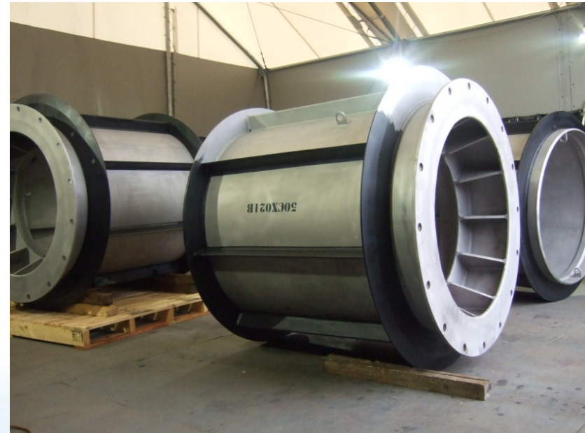
Riser Seat: Manufactured from 6Mo CS Stiffeners/Rings for Interface with Hull
